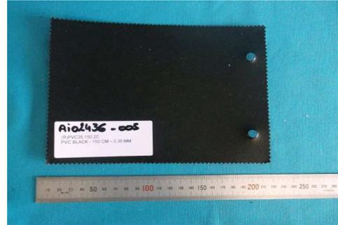
**CONDITIONNEMENT / conditioning of the test specimens**
